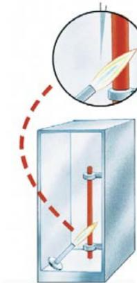
A 60 cm long piece of cable is exposed to a flame for 60 seconds. The cable must not ignite.
