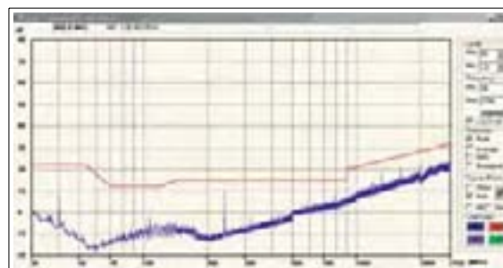
Fig. 13: Shielding attenuation of an HSD connection measured by a stripline setup to CISPR 25
