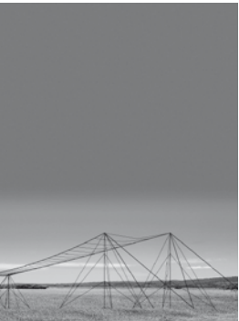
Horizontal and vertical log periodics
